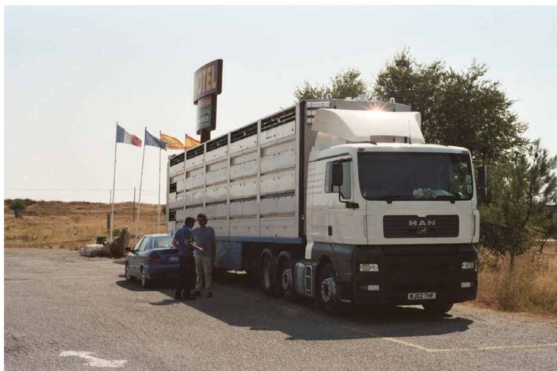
Figure 10. Vehicle configuration – upper deck naturally ventilated, middle and lower deck naturally ventilated.
